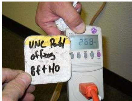
Existing older HO fixture wattage test
