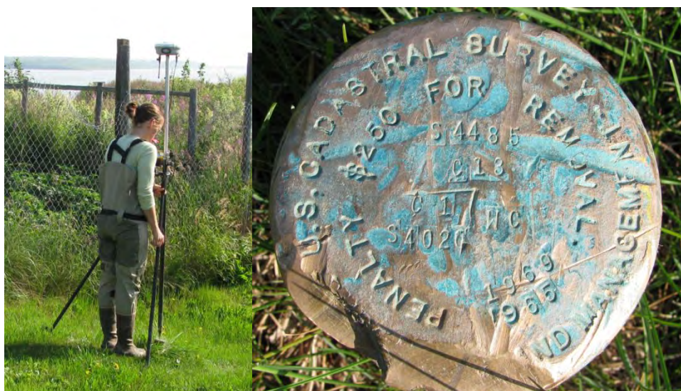
Figure 14: Survey team locating local permanent control monuments (Butterer, 2009).
