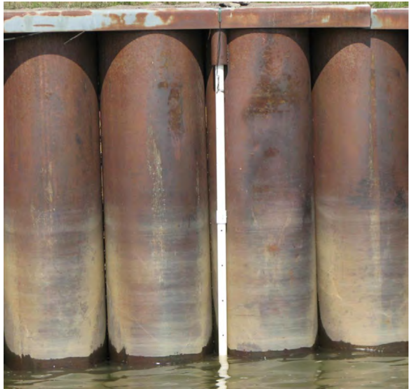
Figure 12: HOBO water level gauge deployed on seawall at Bethel, AK (Yager, 2009).
