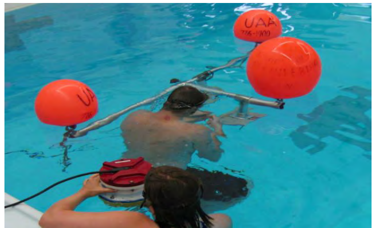
Figure 9: Research members prepare the ADCP for a trial run in the UAA pool (Yager, 2009).
