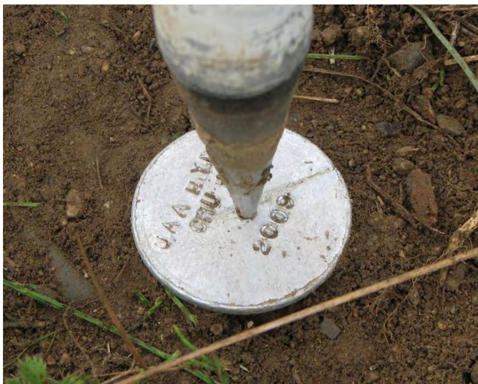
Figure 11: 2 inch aluminum cap set flush to ground on rebar at Chuathbaluk, AK (Harper, 2009).
