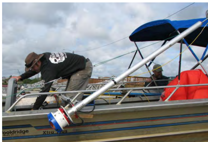
Figure 6: UAA-SOE ADCP side mount fitted to research vessel (Yager, 2009).
